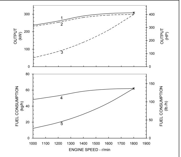
Rating Conditions: Ratings are based upon ISO 8665 and SAE J1228 reference conditions; air pressure of 100kPa [29.612 in.Hg] air temperature 25°C [77°F] and 30% relative humidity.Power is rated in accordance with IMCI
