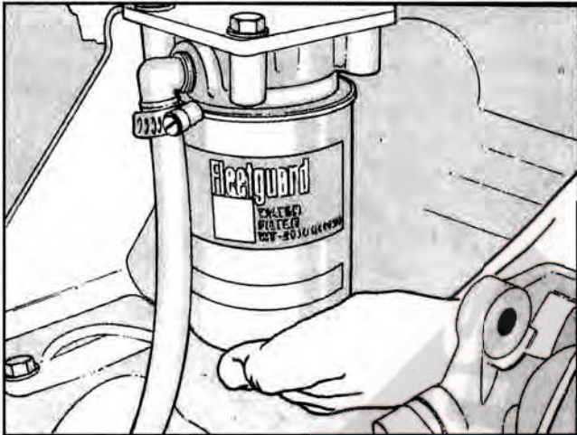
Fig. 2-19 (OM 10236). Installing DCA water filter cartridge
