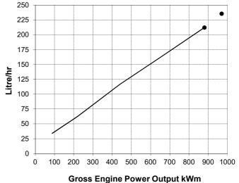
Rating Conditions: Ratings are in accordance with ISO 15550 and ISO 8528-5 reference conditions; air pressure at 100 kPa (29.61 in Hg), air temperature 25°C (77°F), and 30% relative humidity. The fuel consumption data is based on No. 2 diesel fuel weight at 0.85 kg/liter (7.1 lb/U.S. gal).
