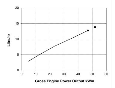
Rating Conditions: Ratings are in accordance with ISO 15550 and ISO 8528-5 reference conditions; air pressure at 100 kPa (29.61 in Hg), air temperature 25°C (77°F), and 30% relative humidity. The fuel consumption data is based on No. 2 diesel fuel weight at 0.84 kg/liter (7.1 lb/U.S. gal).
