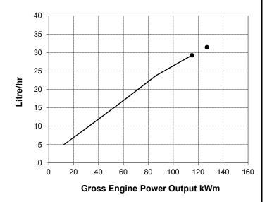
Rating Conditions: Ratings are in accordance with ISO 15550 and ISO 8528-5 reference conditions; air pressure at 100 kPa (29.61 in Hg), air temperature 25°C (77°F), and 30% relative humidity. The fuel consumption data is based on No. 2 diesel fuel weight at 0.84 kg/liter (7.1 lb/U.S. gal).
